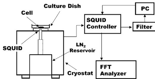
**Figure 5.** A schematic layout of the system. The SQUID was operated in a flux-locked loop with a flux modulation frequency of 256 kHz. The sample in the plastic culture dish was placed on the top of the vacuum window. The signal output was coupled to an A/D interface board and stored in a PC.
