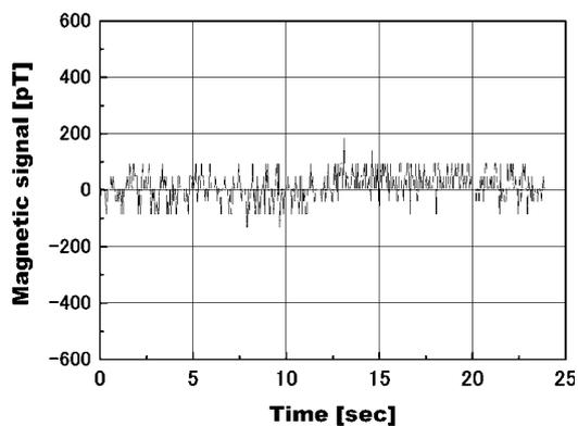
**Figure 7.** Time domain signal trace of the culture dish without cells (blank). A noise level of 30–40 pT was found in the period.
