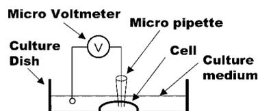
**Figure 1.** Patch clamp method. It is possible to find the growth stage by reading the voltmeter corresponding to the membrane potential of the cell. Using this method, much skill is required to insert the micropipette.
