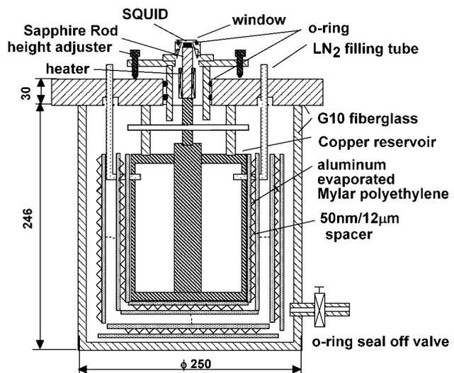
**Figure 4.** Cross-sectional view of the cryostat. This is specially designed for a SQUID microscope. The minimum separation between the SQUID and the sapphire window is  $200\ \mu\text{m}$ .
