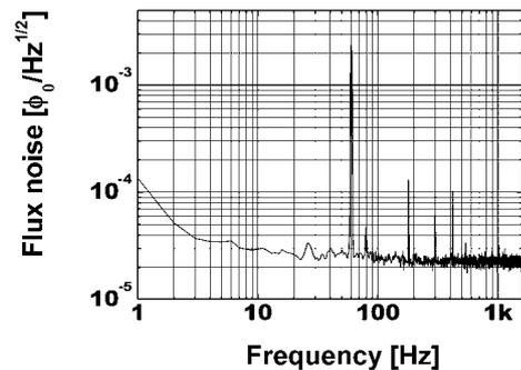
**Figure 3.** Spectral density of flux noise in the SQUID including the electronics. The white noise is about  $20\ \mu\phi_0\ \text{Hz}^{-1/2}$ , which corresponds to  $0.36\ \text{pT}\ \text{Hz}^{-1/2}$ .
